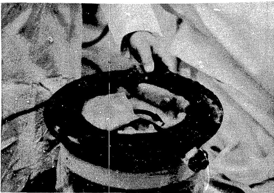
Figure 16. Stainless Steel Container Rim. The lid has just been removed. Notice how "dirty" the rim area which was under the gasket is. The radiation level measured 3 mR/hr in approximately the probe location shown in the photograph.
